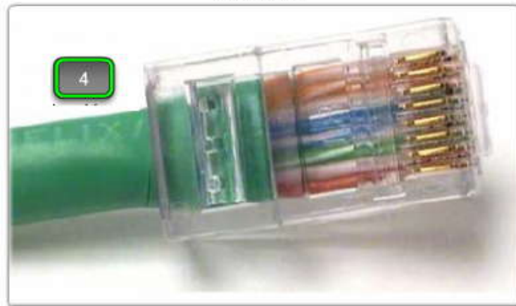
Cable Ethernet TIA/EIA 568B UTP.
